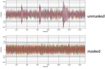
→ No more 1<sup>st</sup> order leakage with this masking scheme.
