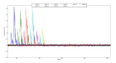
In the **worst case scenario** (profiled attacks), these can be **combined** with other leakage points later to perform a **second order attack**. (M; SBOX(P $\oplus$ K) $\oplus$ M)  $\Rightarrow$  SBOX(P $\oplus$ K)
