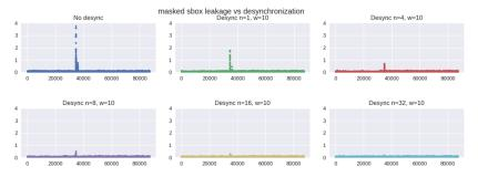
→ Leakage shrinks and becomes **unexploitable** (20000 traces here).
