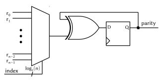
Fig. 10: Hardware architecture of the parity computation module when multiplexing the response bits stored in registers.
