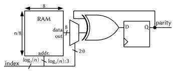
Fig. 12: Hardware architecture of the parity computation module where the PUF response is stored in RAM
